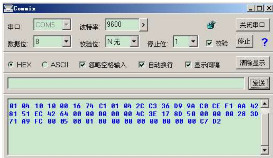
Figure 6-5 Example of Serial Port Debugging Assistant Listening
