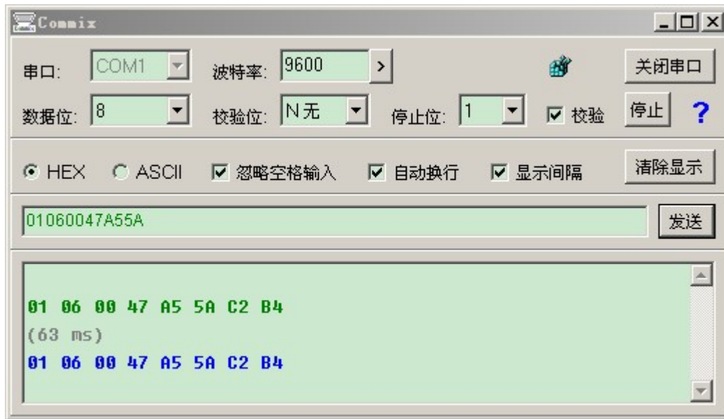
Figure 4-1 Total Zeroing Frame Structure
