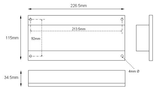
If using HDA0002 DIN rail adapter brackets the overall depth from the gear plate to the front surface of the device is 45.5mm
