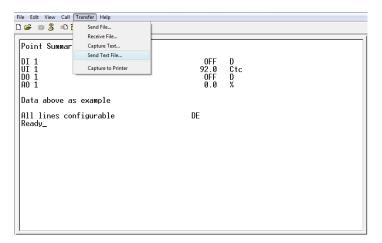
After the text file has downloaded you will briefly see a check of the number of lines expected versus the number of lines received. If the two values are equal 'Restarting...' will be displayed at which point the new configuration is written to non-volatile memory automatically.
