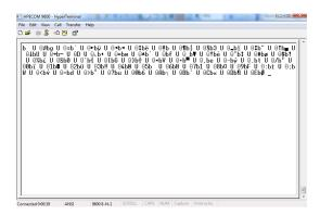
To break in to terminal mode set Caps Lock on and hold the 'T' character key continuously (TTTTTTT...). After five (5) T's have been sent to the device it will switch to terminal mode. At this point the BACnet activity on the network will be halted and the device will display the default user screen.
