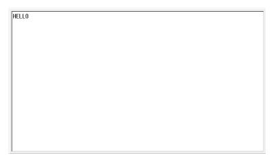
To break in to terminal mode set Caps Lock on and hold the 'T' character key continuously (TTTTTTT...). After five (5) T's have been sent to the device it will switch to terminal mode. At this point the device will display the default user screen.
